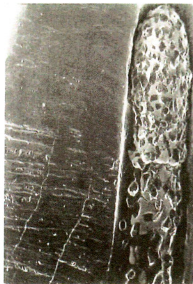
Figure 8. SEM of 2-Grit diamond showing fine grit at tip with corresponding smooth enamel, and coarse grit on shank with deeper striations on enamel.
