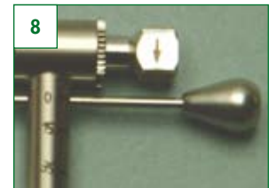
8 Directional arrow must be pointing clockwise (towards torque bar with tear drop). If not, pull arrow out, flip over, and push back in.
