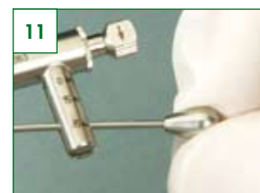
11 Grasp only the tear drop and move the torque bar to the 35 Ncm mark.
